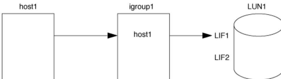
You can limit access to LUN1 by using a port set. In the following example, initiator1 can access LUN1 only through LIF1. However, initiator1 cannot access LUN1 through LIF2 because LIF2 is not in port set1.
